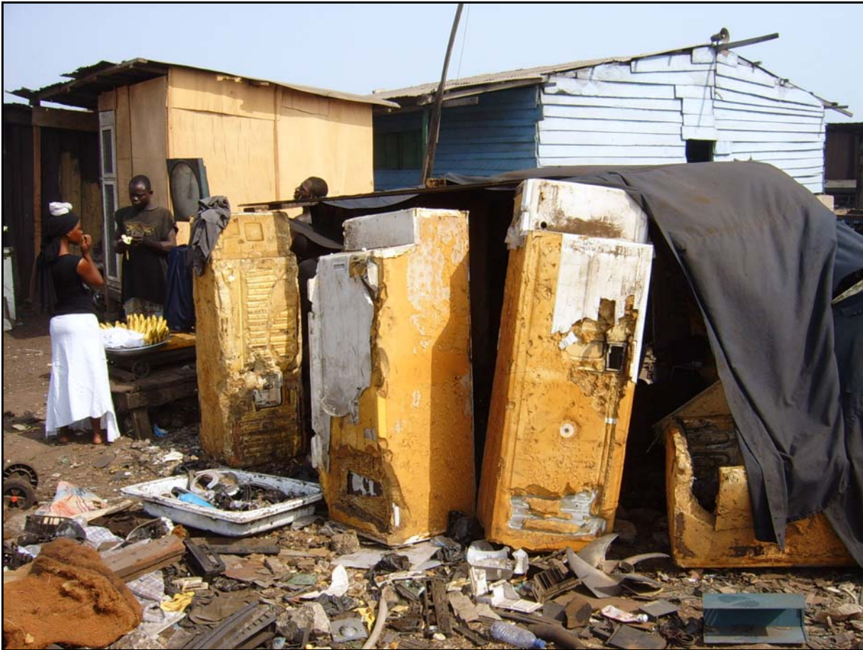
Photo 10 Corpuses of refrigerators after manual extraction of steel, copper and aluminium (Source: Öko-Institut 2010)
