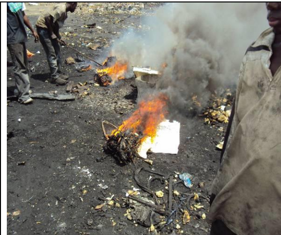
Burning of cables to extra copper from them.
