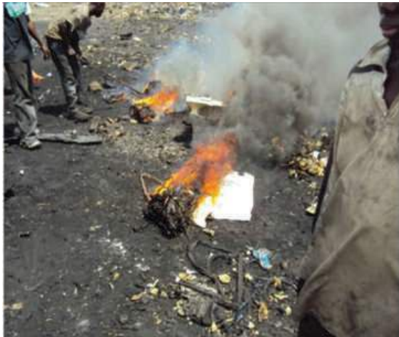
Burning of Cables to Extract Copper
