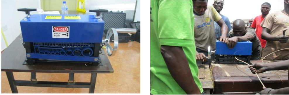
**Fig.3 Cranker on a Table (Left) and Workers using Cranker to Strip a Cable (Right)**
